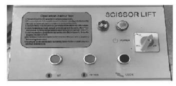
When the power supplied, turn the *POWER SWITCH* clockwise while the machine is on standby and an *INDICATOR* will show.
